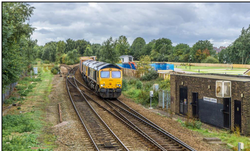
above: GBRF 66722 'Sir Edward Watkin' passes Mexborough Jn with a Rotherham-Felixstowe intermodal on 12 Sept. 2017. The single line to Kilnhurst and Aldwarke goes off to the left. In the past the lines towards Wath quadrupled at this point and the Kilnhurst line was double-track with sidings alongside, all controlled by Mexboro No.2 box located to the left of this view.
