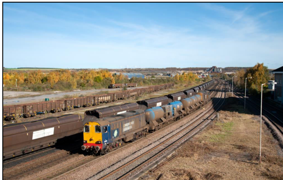
below: DRS 20305+20302 head towards Scunthorpe station with the RHTT on 27 October 2017. These trains soon acquire a coating of grime thrown up from the track when the spray is operating. Viewed from Brigg Road bridge looking east. There are just over two miles of quadruple track extending from Santon to Scunthorpe station. Part of the iron ore storage and blending plant at Santon can be seen in the distance.
